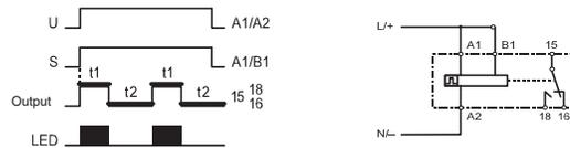
Pulse Controlled, Output Starts With Pause (Min. Pulse AC 50 ms — DC 30 ms) — Switch ⊗ is Up One Cycle Mode — Voltage Supplied at A1 and A2, then Pulsing "s" to Energize B1 will Initiate One Cycle.
