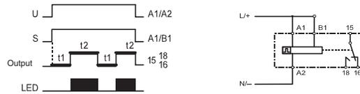
Supply Voltage Controlled, Oscillating Mode Starting with Pulse — Switch ⊗ is Down
