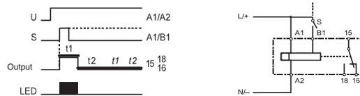
**Note:** If B1 is pulsed, a one full time cycle consisting of  $t_1$  and  $t_2$  is completed.
