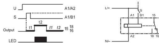
Pulse Controlled, Output Starts with Pulse (Min. Pulse AC 50 ms — DC 30 ms) — Switch ⊗ is Down One Cycle Mode — Voltage Supplied at A1 and A2, then Pulsing "s" to Energize B1 will Initiate One Cycle.
