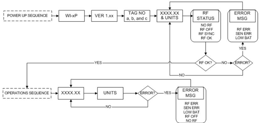
Figure 4.1: Field Unit Power-Up and Operations LCD Sequences
