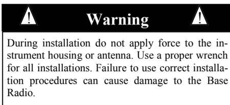
Give careful consideration to the environment where you will be installing your instrument. Avoid installations that expose the device to excess temperature, high vibration, considerable shock, or exposure to dripping condensate or corrosive materials. Also avoid installing the device in an un-serviceable location.
