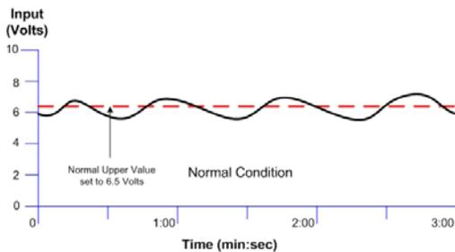
Figure 6.13: Condition "Chatter" Elimination Due to Time Deadband
