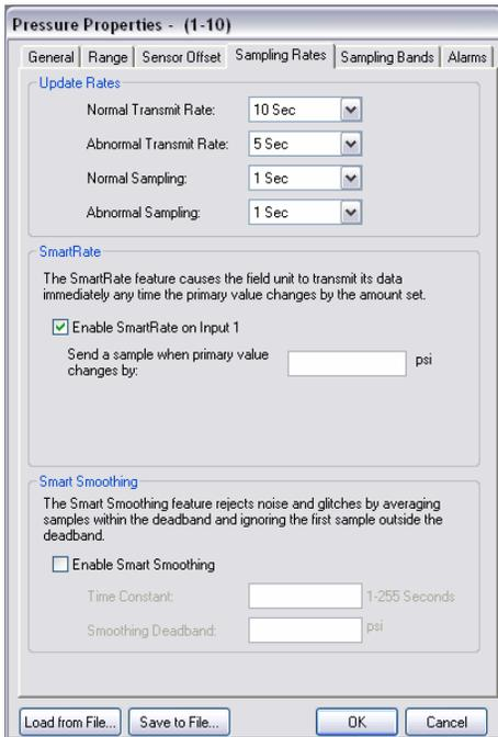
Figure 6.9: Smart Rate Configuration Using Wireless Instrumentation Manager
