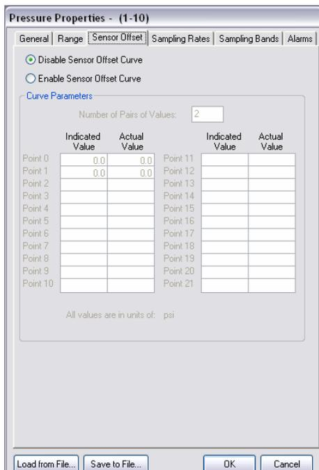
If you have the Wireless Instrumentation Manager software, a 22-point sensor offset curve may be entered for the Field Unit. To do so, enter the configuration menu (See Section 9.2 of the Wireless Instrumentation Manager User Manual). Once in the configuration menu click on the **Sensor Offset** tab to bring up the offset information as shown in Figure 7.6.
