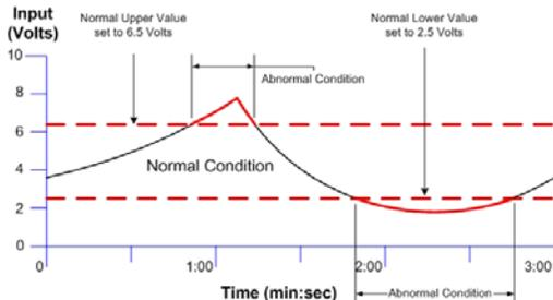
Figure 6.10: Normal Upper and Lower Value Example
