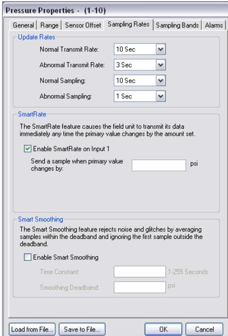
Figure 6.14: Sampling and Transmission Rate Selection Using the Software
