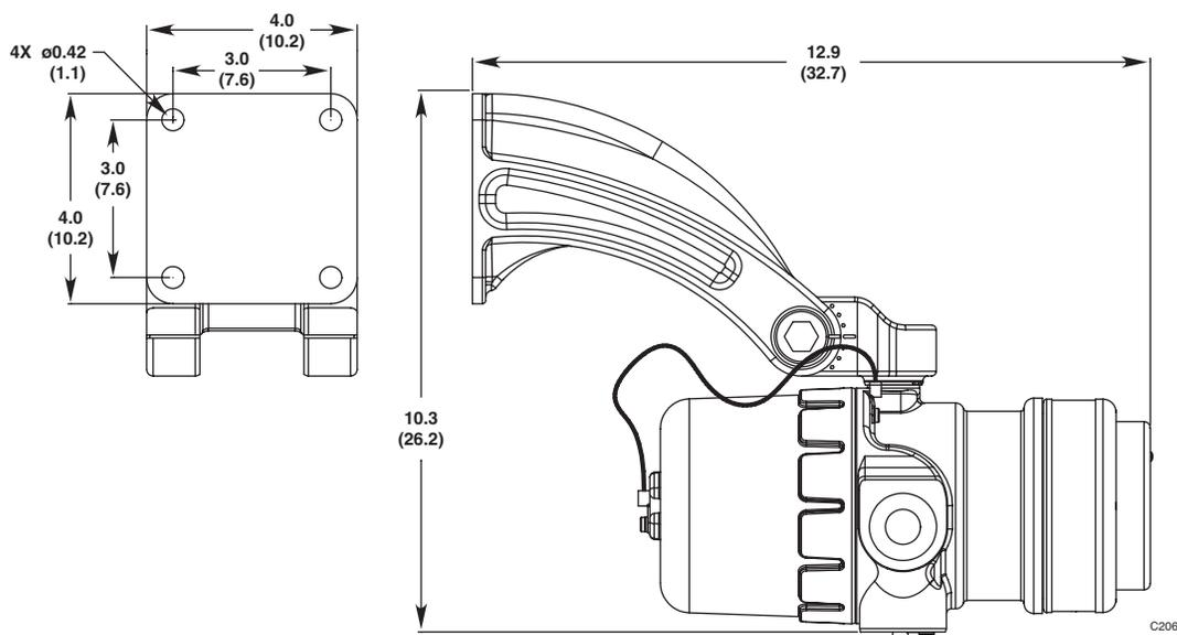
Figure 3—Q9033B Mounting Bracket Dimensions in Inches (cm)
