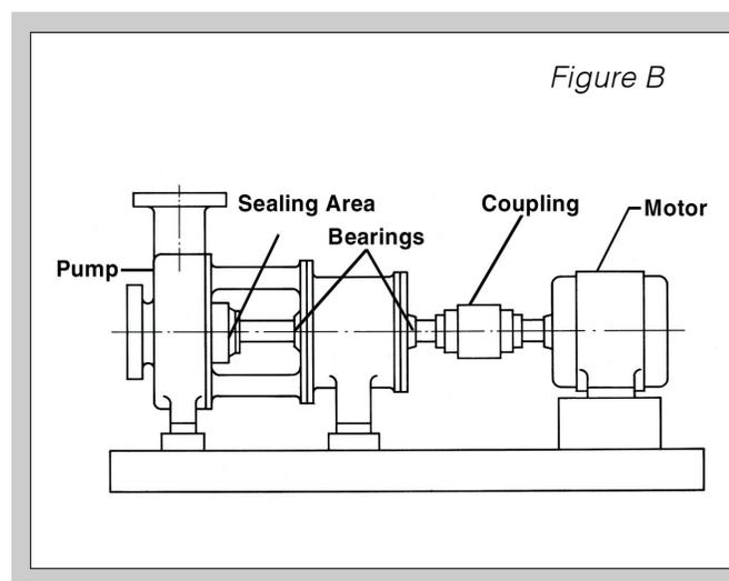
Dynamic seals are frequently located on the shaft of a centrifugal pump. The pump converts the electric motor's rotating energy into velocity, or pressure energy of the liquid or gas being moved.
