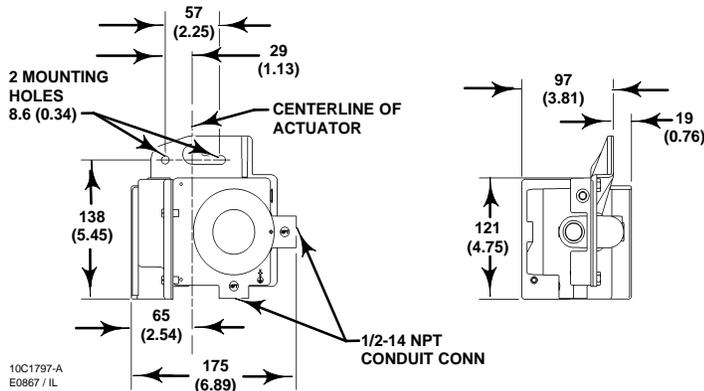
**TYPE DVC6015 SLIDING STEM ACTUATOR MOUNTING
