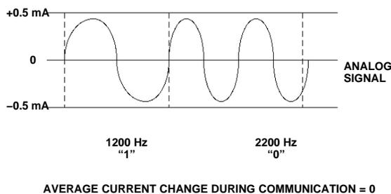
Figure 8. HART® Frequency Shift Keying Technique
