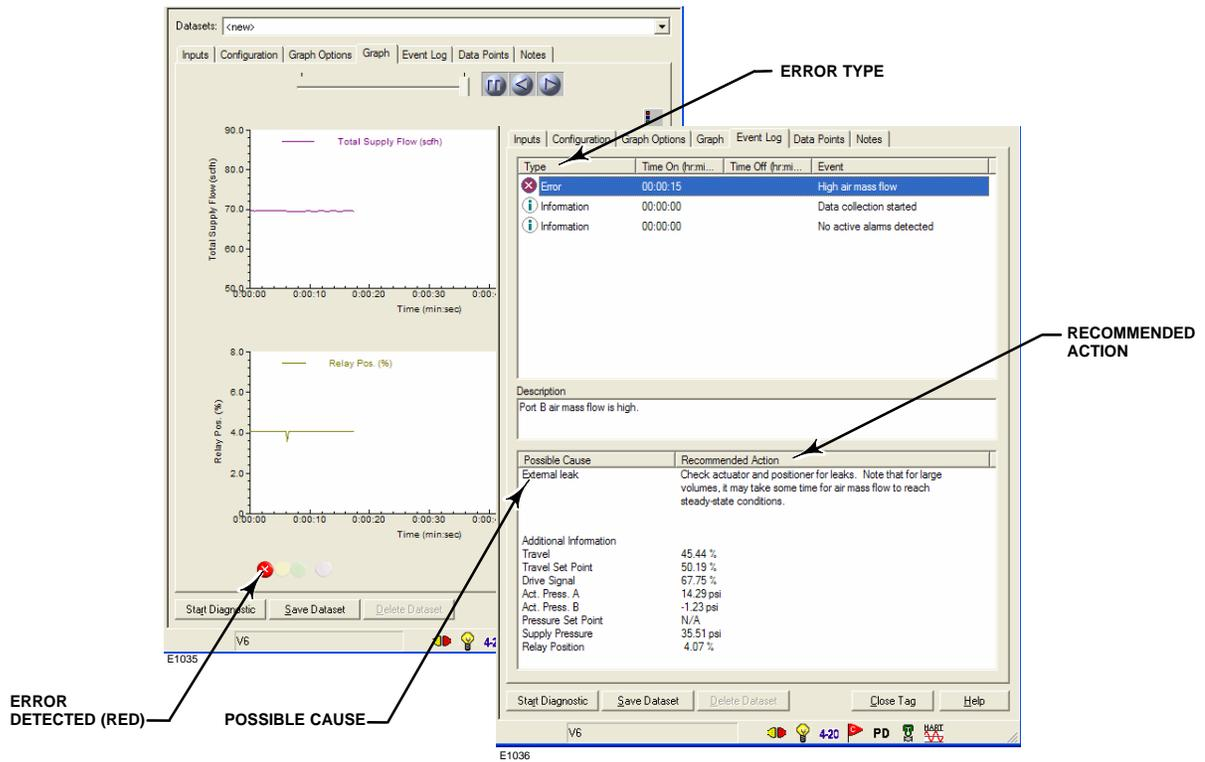
Figure 4. One-Button Sweep—Air Mass Flow Diagnostic
