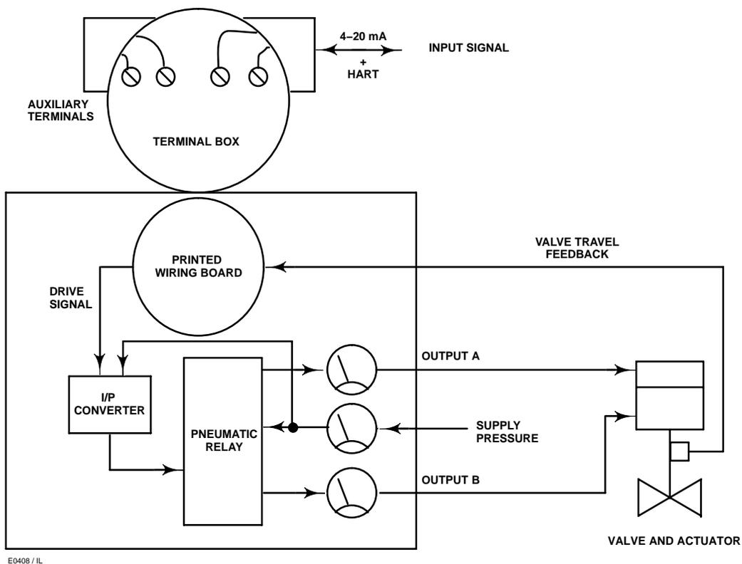
Figure 11. DVC6000 Series Digital Valve Controller Block Diagram
