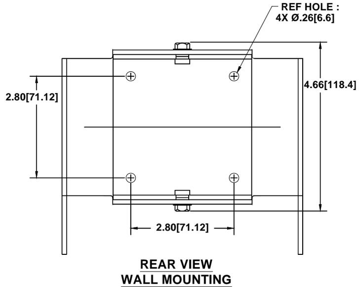
Figure 10: 71072 Mounting Bracket Drawing (Class I, Div 1 & 2, Groups B, C & D or Zone 1 and 2)
