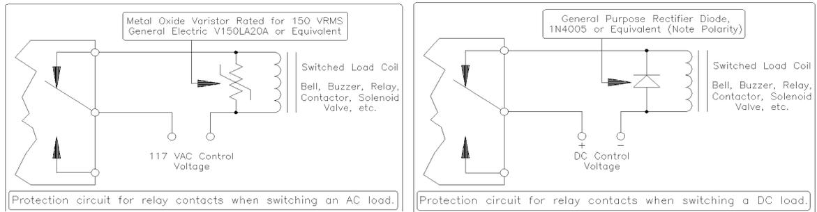
**Figure 7 Relay Contact Protection for AC/DC Loads**
