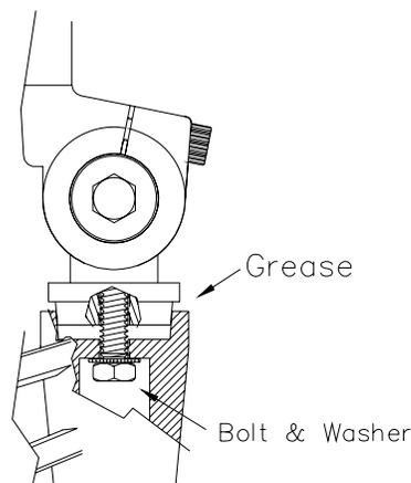
**Figure 17 System Mounting Hardware**
