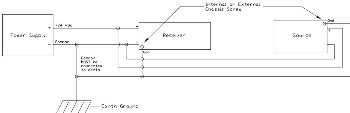
**Figure 30 Grounding Connections**
