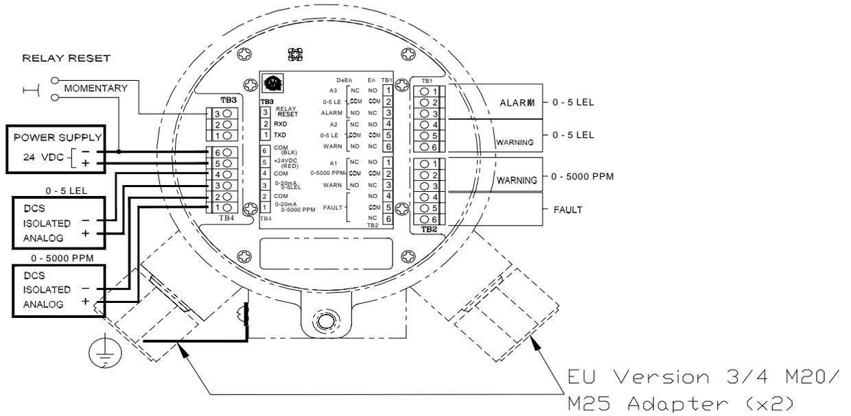
**Figure 24 European Union IR Receiver Terminal Block Location**
