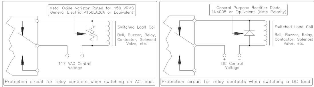
**Figure 20 Relay Contact Protection for AC/DC Loads**
