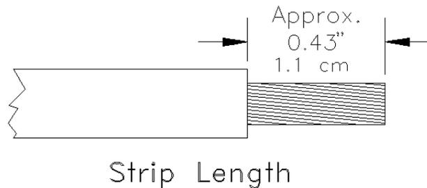
**Figure 19 Wire Strip Length Diagram**
