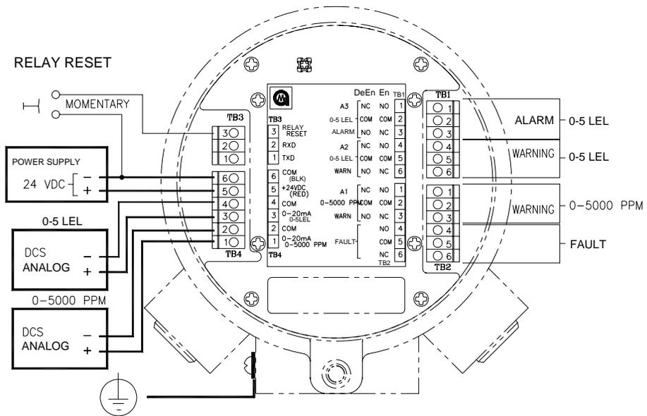
**Figure 23 IR Receiver Terminal Block Location /Standard Unit Shown**
