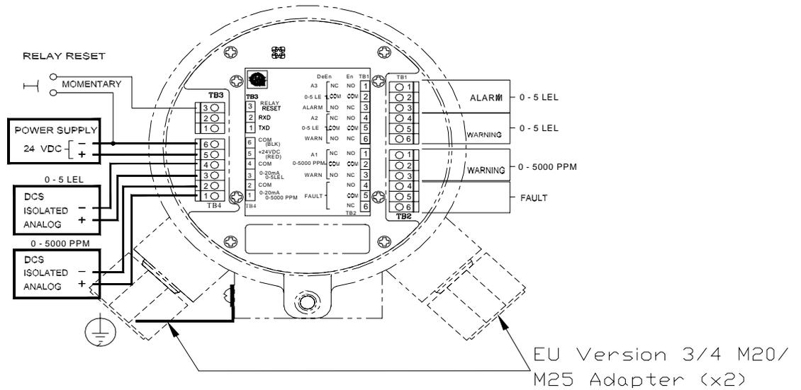
**Figure 11 European Union Receiver - Terminal Block Location**
