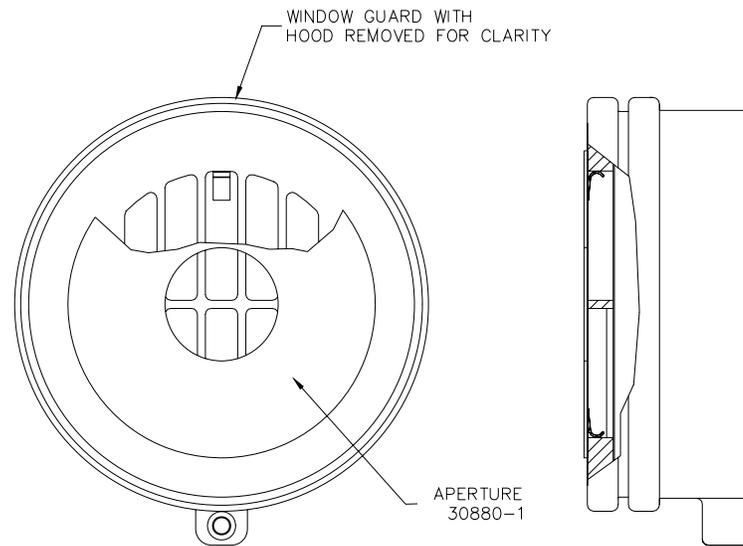
ALIGN APERTURE PLATE OVER GUARD AND PRESS INTO PLACE
