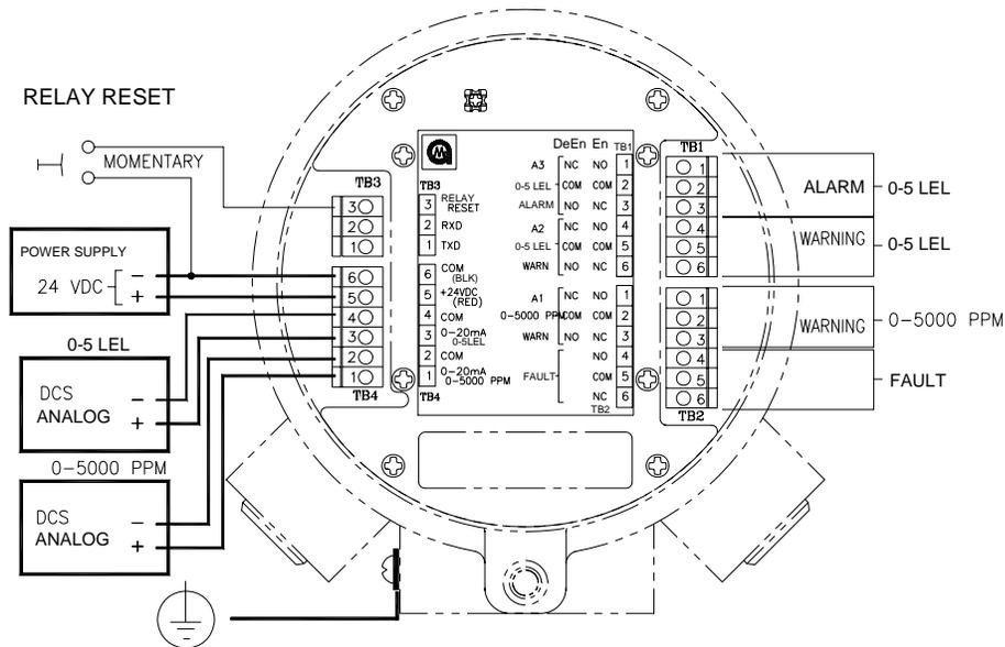
**Figure 10 Receiver - Terminal Block Location**
