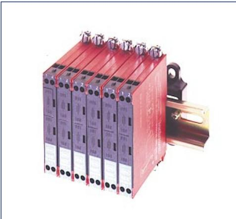
**Multiple barriers mounted to 35mm DIN Rail. Each barrier occupies 1/2" of rail space. Once mounted the barrier forms an electrical connection with the rail which now serves as the intrinsic safety ground bus.**
