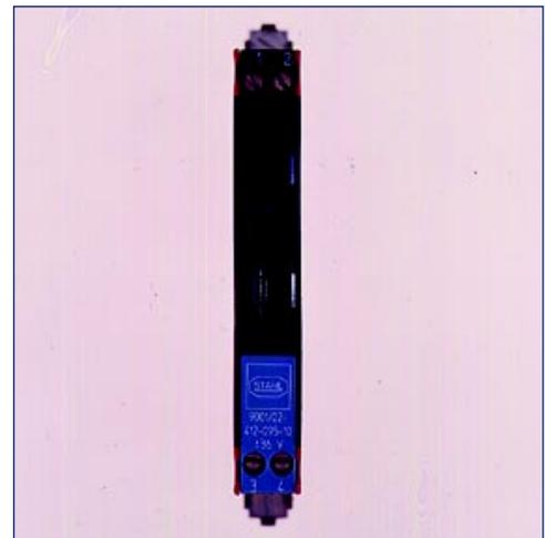
Top view of safety barrier showing screw terminal connections for both safe and hazardous area terminations. The replaceable fuses are contained in recessed compartments and are interchangeable with all Series 9000 INTRINSPAK.
