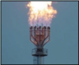
Flare gas exiting the INDAIR flare tip entrains and turbulently mixes 20 times its volume of air as it travels around the tulip-shaped Coanda profile.
