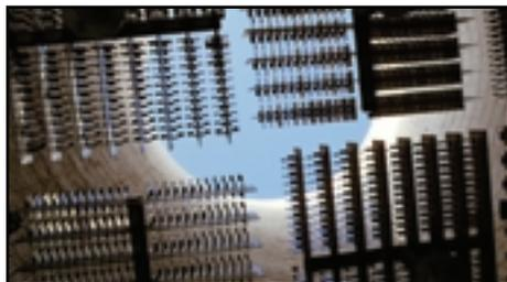
*The thin, "tear drop-shaped" gas distribution manifold of the fin plate burner provides a large open area for combustion air entrainment.*
