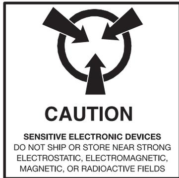
Magnetrol's electronic instruments are manufactured to the highest quality standards. These instruments use electronic components that may be damaged by static electricity present in most work environments.
