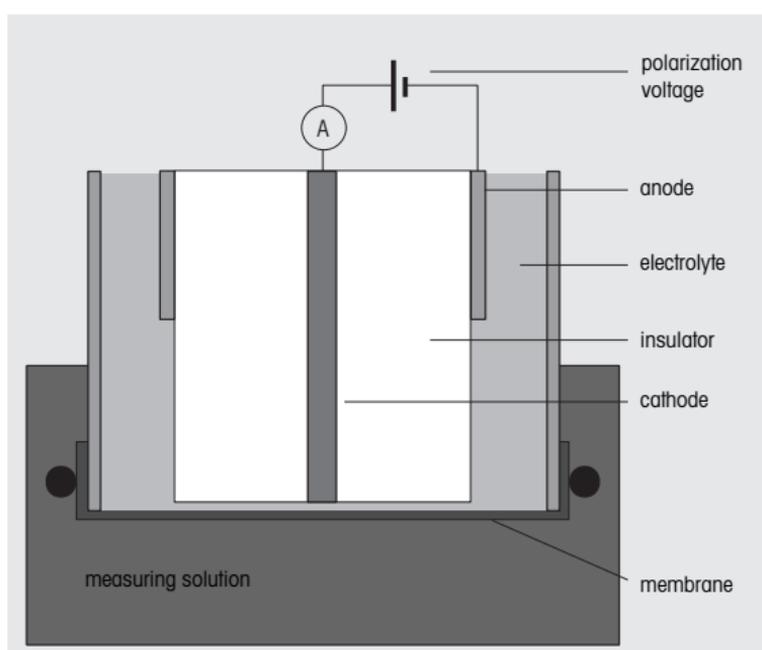
In the case of the Clark electrode, geometrical configuration is very important. In particular, the thickness of the electrolyte film between the cathode and the membrane must be within narrow tolerances so as to ensure good linearity and a low zero current (current in a nitrogen atmosphere). The figure above exemplifies the principle of the design of a Clark-type oxygen electrode.
