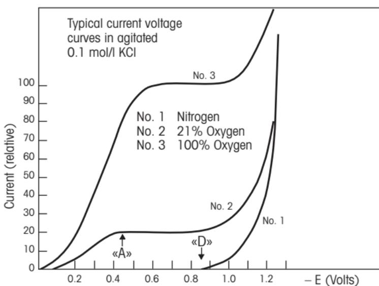
The polarization voltage should remain as constant as possible. Besides a constant source of voltage the following prerequisites must be met:
