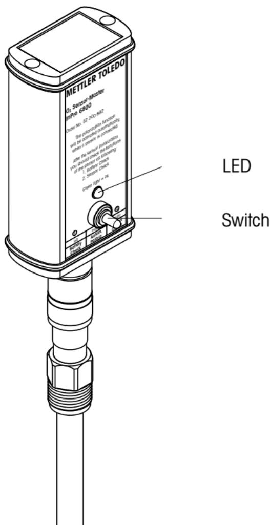
As soon as the sensor is connected to the O<sub>2</sub> Sensor-Master, the polarization function is automatically activated. Please note: if the sensor was disconnected from the transmitter for longer than 5 minutes, the sensor must be polarized first (polarizing time see section 5.1) to get representative test results.
