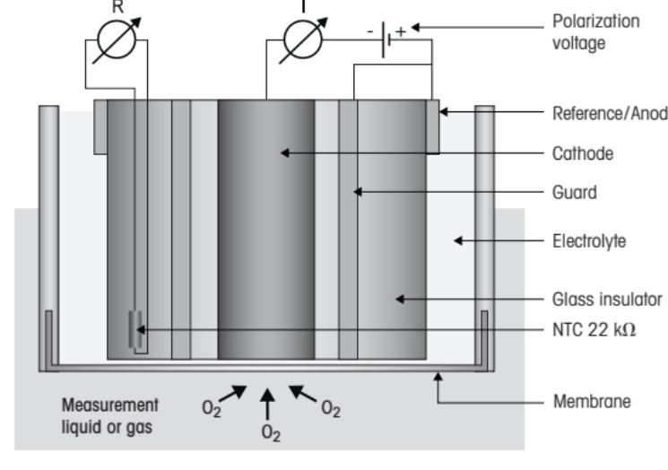
In all sensors the function of the cathode is identical.
