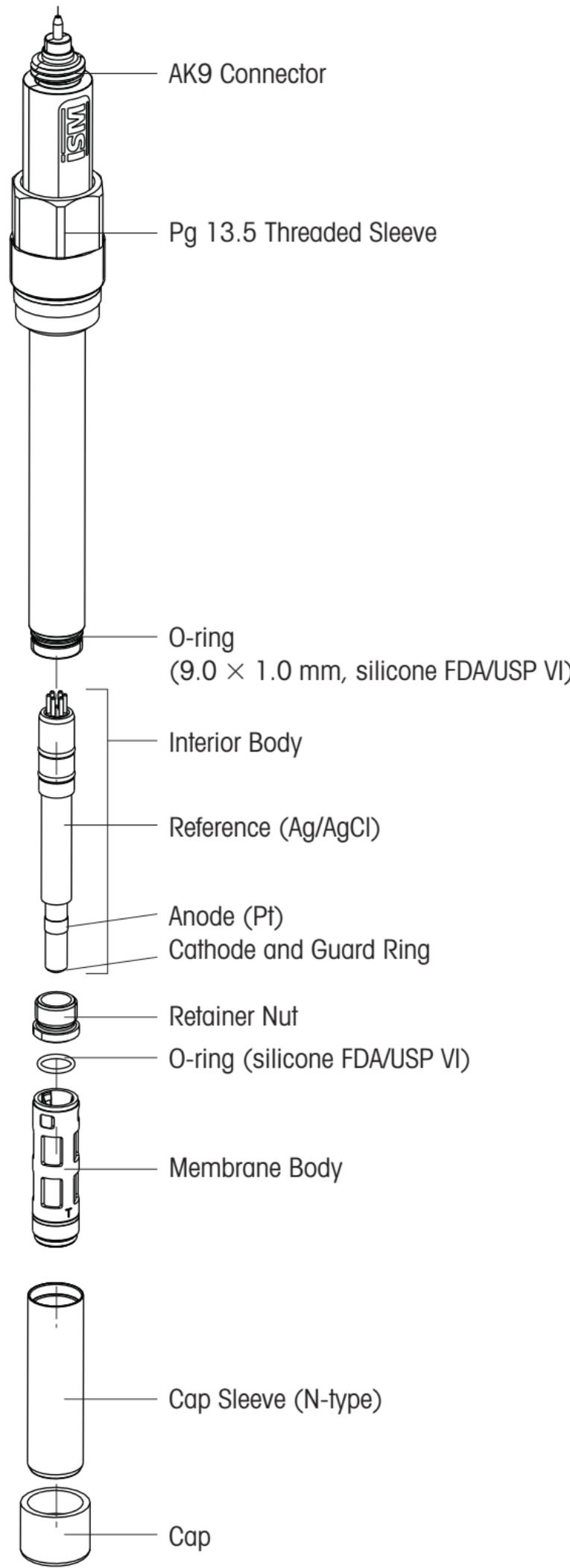
METTLER TOLEDO DO sensors are supplied with fitted membrane body but without electrolyte and covered with the protection cap and have been checked for proper function.
