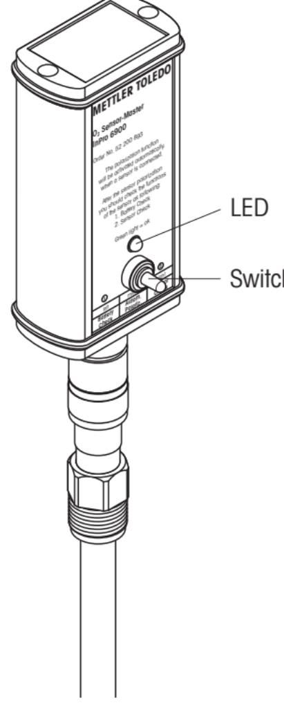
As soon as the sensor is connected to the O<sub>2</sub> sensor master, the polarization function is automatically activated. Please note: if the sensor was disconnected from the transmitter for longer than 5 minutes, the sensor must be polarized first (polarizing time see "Section 5.1") to get representative test results.
