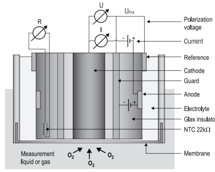
As a consequence of the reaction at the cathode and the anode, a current flows between cathode and anode (4 electrons per oxygen molecule), which is proportional to the oxygen partial pressure at the cathode.
