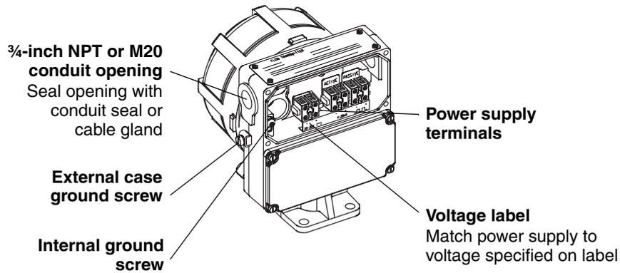
7. Make sure the power cable is not installed in the same conduit or cable tray as output wiring.
