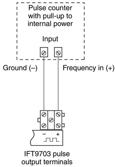
**Figure 3-7** Wiring to pulse counter without internal pull-up resistor
