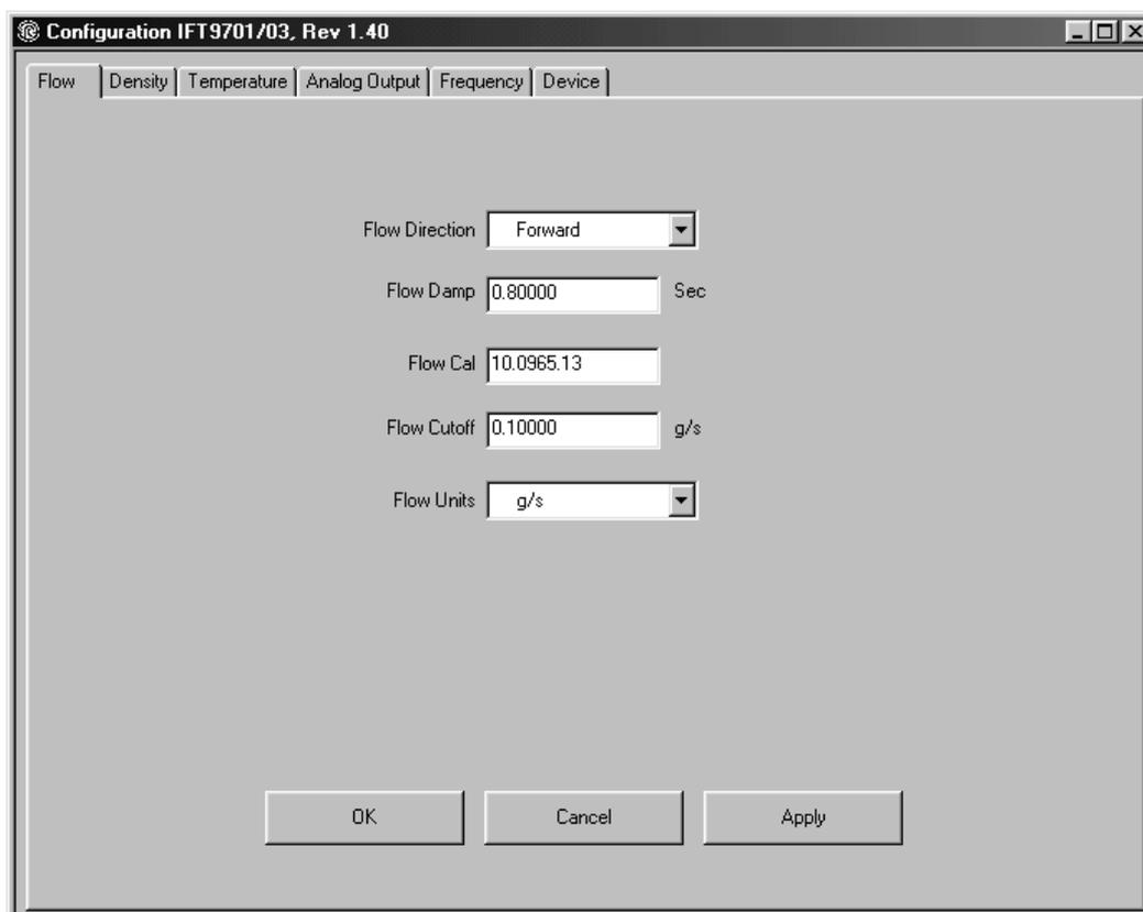
3. To specify the flow measurement unit, open the Flow Units list box and select a flow unit. If you select a unit of mass flow, the transmitter will measure mass flow. If you select a unit of volume flow, the transmitter will measure volume flow. A list of available flow measurement units is provided in Table 6-1.
