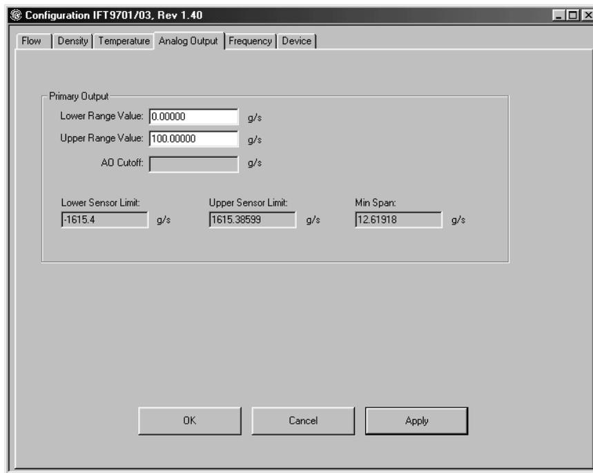
3. Range values are flow rates represented by the milliamp output at 4 mA and at 20 mA. To set range values:
