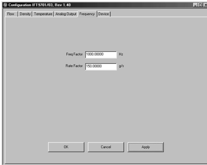
3. The pulse output produces a frequency proportional to the flow rate. Pulse output scaling requires entry of frequency and flow rate values. To scale the pulse output:
