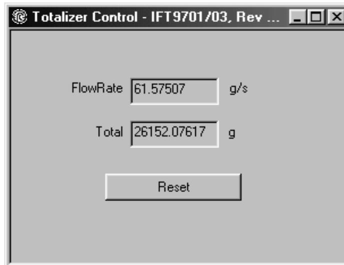
5. Click the Reset button to reset the internal totalizer to zero.
