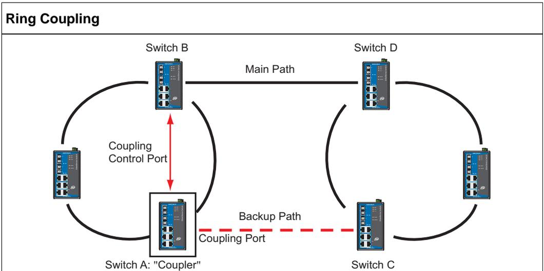
To support the Ring Coupling function, select two EDS-508A/505A (e.g., Switch A and B in the above figure) in the Turbo Ring and another two EDS-508A/505A in the adjacent Turbo Ring (e.g., Switch C and D).
