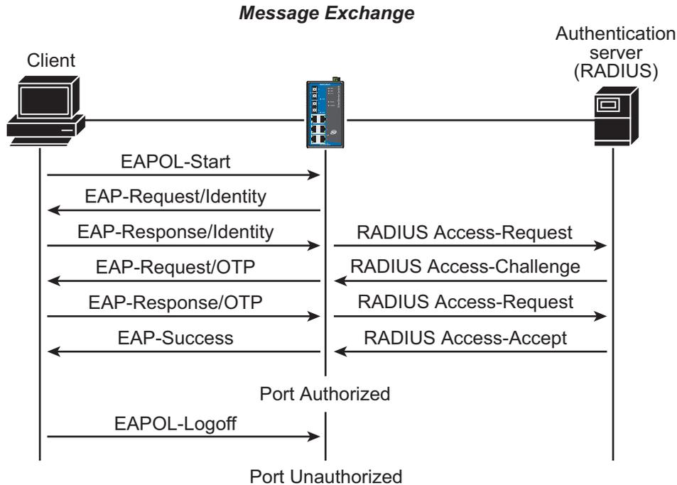
1. When the supplicant receives an “EAP Request/Identity” frame, it sends an “EAP Response/Identity” frame with its username back to the authenticator.
