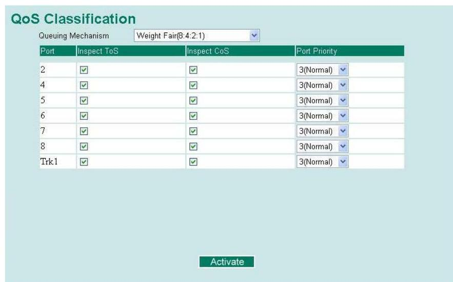
MOXA EDS-508A/505A supports inspection of layer 3 TOS and/or layer 2 CoS tag information to determine how to classify traffic packets.
