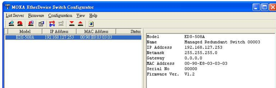
3. Click the **Upgrade Firmware** toolbar icon
