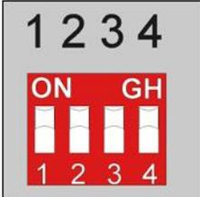
Note: Positions 2 and 3 should only be used in RS422 Mode. Enabling TXD/RTS termination may be required to avoid errors at high bit rates or long cable lengths. The cable is tested up to 1,000 feet but the maximum may be more with termination enable and lower data rates.
