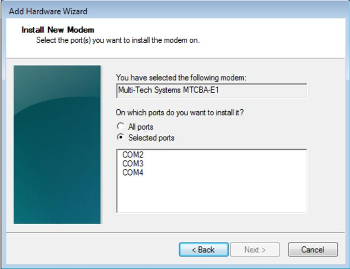
If you know exactly which port your modem is on, click on that port; otherwise, go to **Device Manager > Ports (COM & LPT)** to verify which port the **MultiModem Cell MTCBA-X-U** is installed on. Click **Next**.
