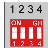
**Note:** Positions 2 and 3 should only be used in RS422 Mode. Enabling TXD/RTS termination may be required to avoid errors at high bit rates or long cable lengths. Multi-Tech Systems tested the cable up to 1,000 feet, but the maximum may be more with termination enabled and lower data rates.
