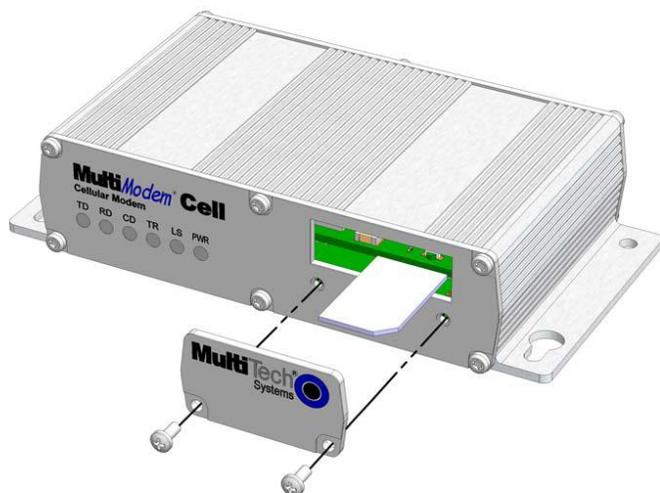
2. Insert the SIM card into the card holder. The above graphic illustrates the correct SIM card orientation.
