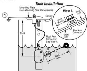
NOTE: When installing the fuel sender in a non-metallic tank using a single wire sender, another wire must be added from one of the sender mounting bolts to the battery ground (negative post). See 1 in the 'Tank Installation' illustration above.
