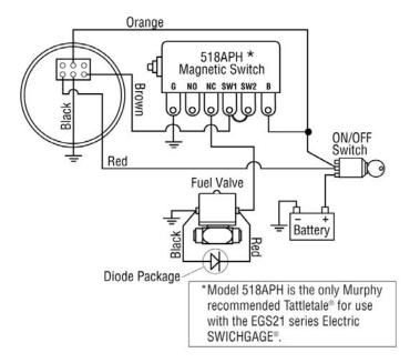
NOTE: Do not connect 117PH or power on TL7 to brown wire. Only use 518(A)PH or 760 Tattletale indicators. Pilot a relay with a flyback diode across the coil for loads pulling more current than rated.
