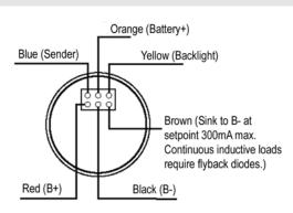
CAUTION: Devices containing solid state components can be damaged or caused to malfunction when used in systems which incorporate inductive loads (e.g. relays, solenoids, etc.) that can generate voltage spikes.
