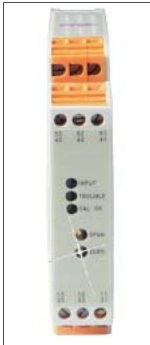
The DRG-SC-TC is a DIN rail mount thermocouple input signal conditioner. It can be field configured for over 60 different thermocouple temperature ranges. The output is linear to temperature and can be set for either 0-5 V, 0-10 V, 0-1 mA, 0-20 mA or 4-20 mA. Zero and span pots allow 50% adjustability of offset and span turn down within each of the ranges. For example the 500-1000°C range could be offset and turned down to provide a 4-20 mA signal representing 750-1000°C.
