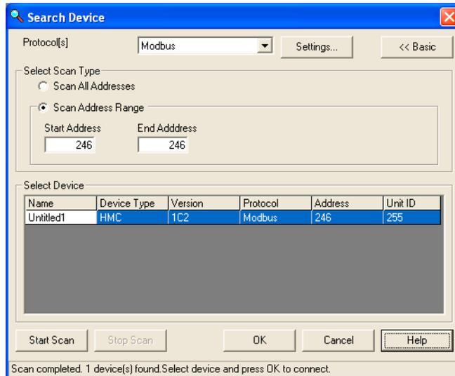
6. Search for HMCs by selecting “Scan Address Range”, and choose a start and end address for Modbus. The default HMC Modbus address is 246.
