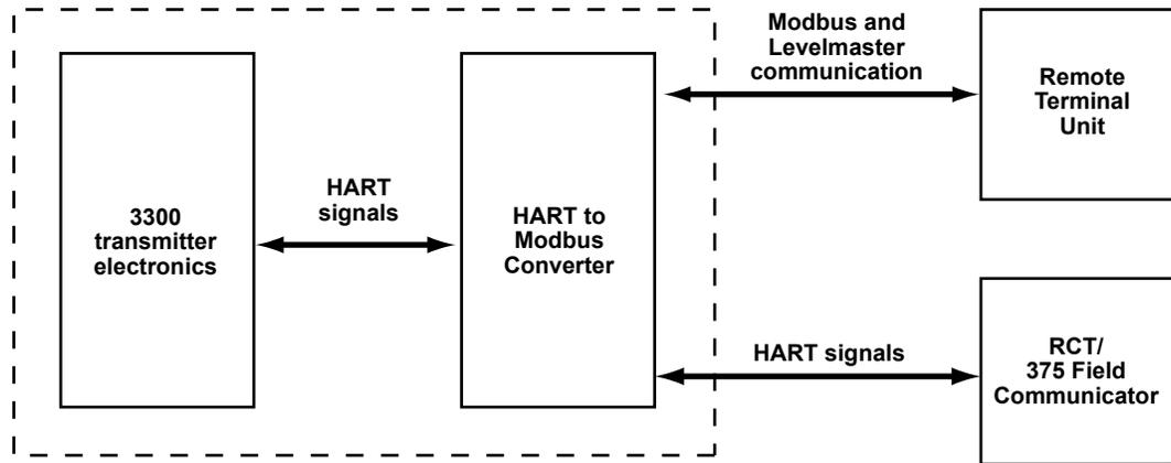
During normal operation, the HMC “mirrors” the contents of process variables from the 3300 transmitter to the Modbus registers. To configure the 3300 transmitter, it is possible to connect a configuration tool to the HMC. See “Transmitter Configuration” on page 1-7 for more information.
