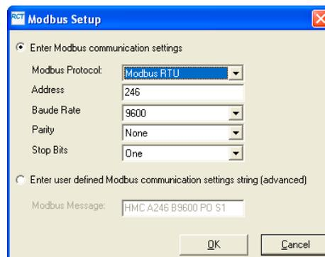
5. In the *Modbus Setup* window, type the desired Modbus RTU address.
