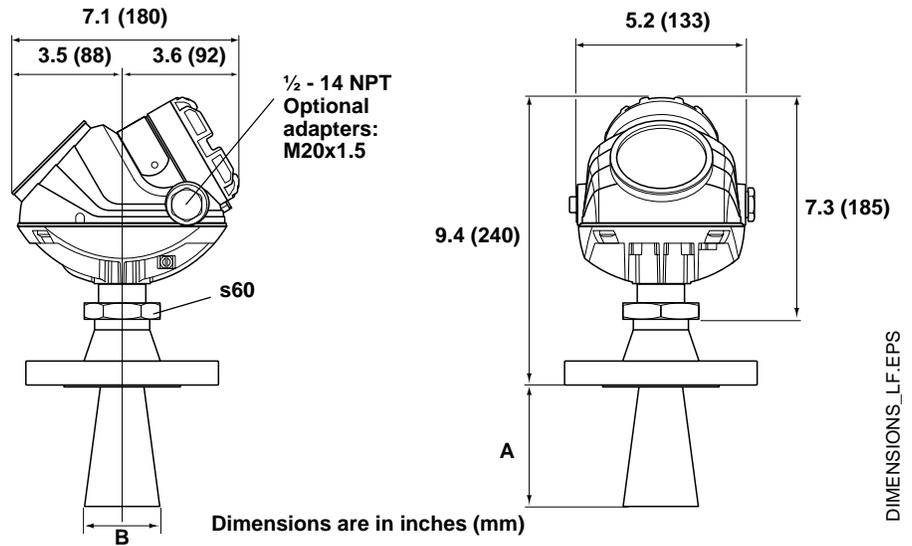
Figure A-3. Model 5402 (High Frequency version) transmitter with cone antenna.
