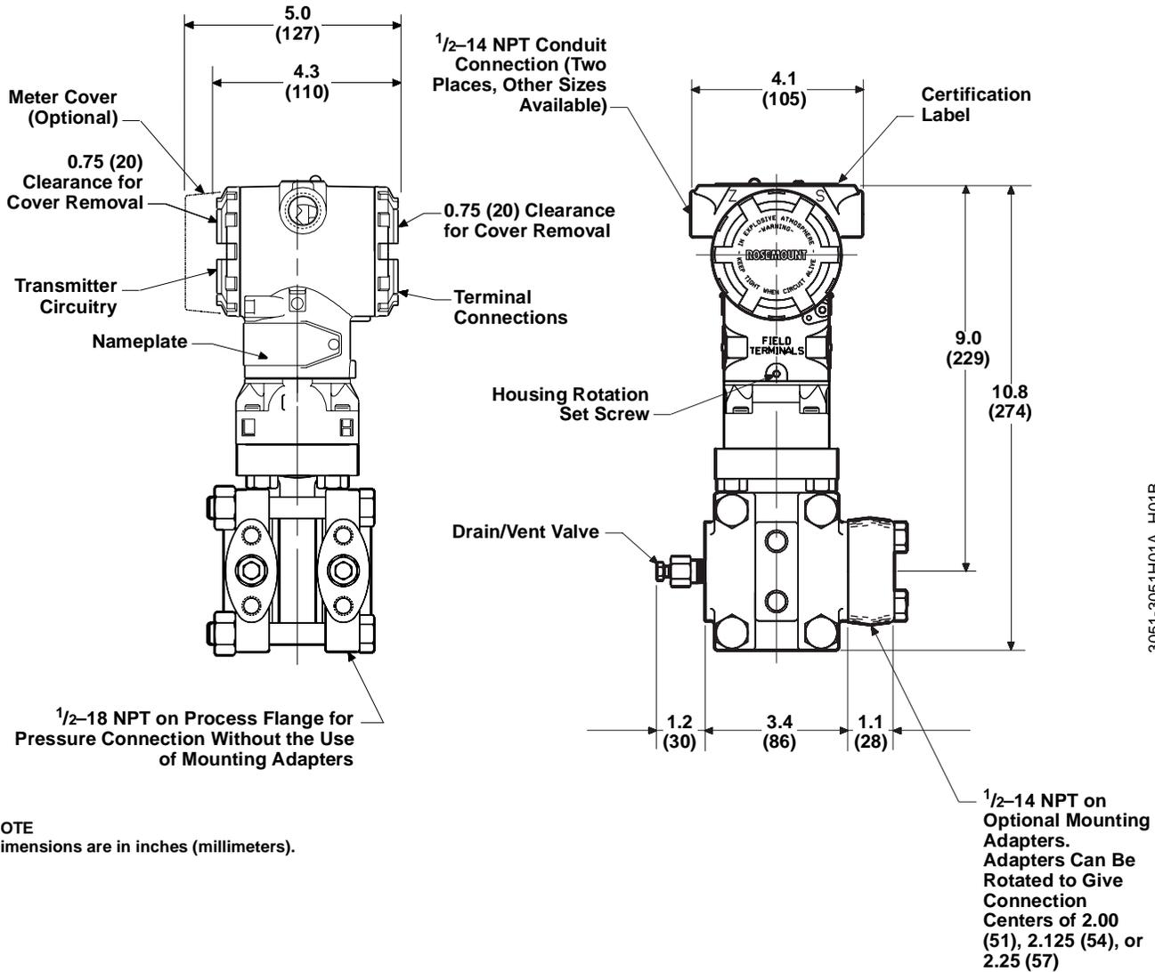
TABLE 3-1. Model 3051L Dimensional Specifications—*Except Where Noted, Dimensions Are in Inches (Millimeters).*
