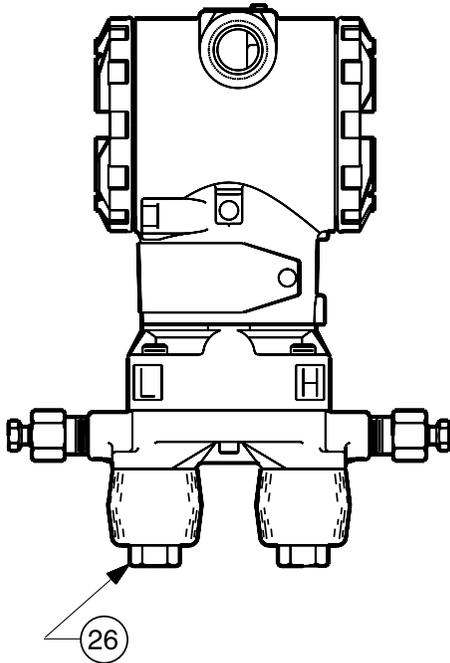
Transmitter with Coplanar Flange, 3-Valve Manifold, and Flange Adapters (Differential Version)
