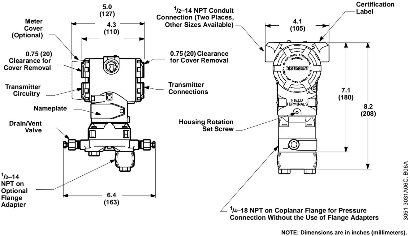
FIGURE 3-4. Model 3051C (Traditional Flange) Dimensional Drawings.
