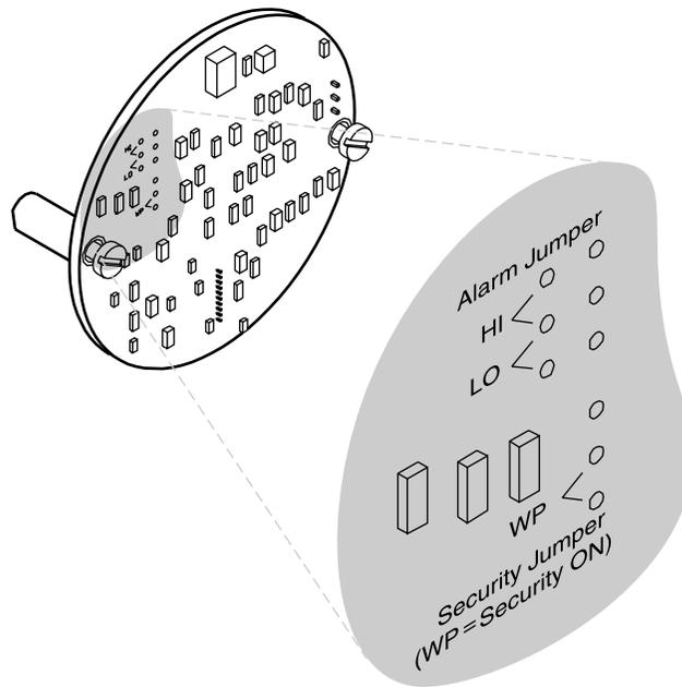
On one version of the previous electronics board, the security jumper is located on the back side of the board. Contact Rosemount Customer Central at 1-800-999-9307 for more information.
