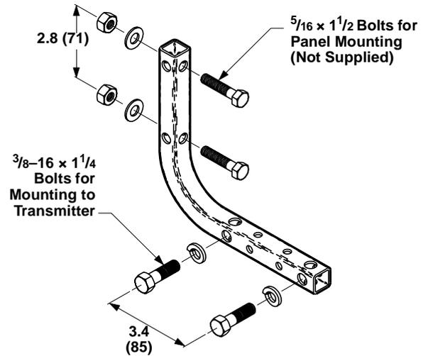
Panel Mounting Configuration 3/8-16 x 1 1/4 Bolts (2) Supplied for Attaching Bracket to Transmitter
