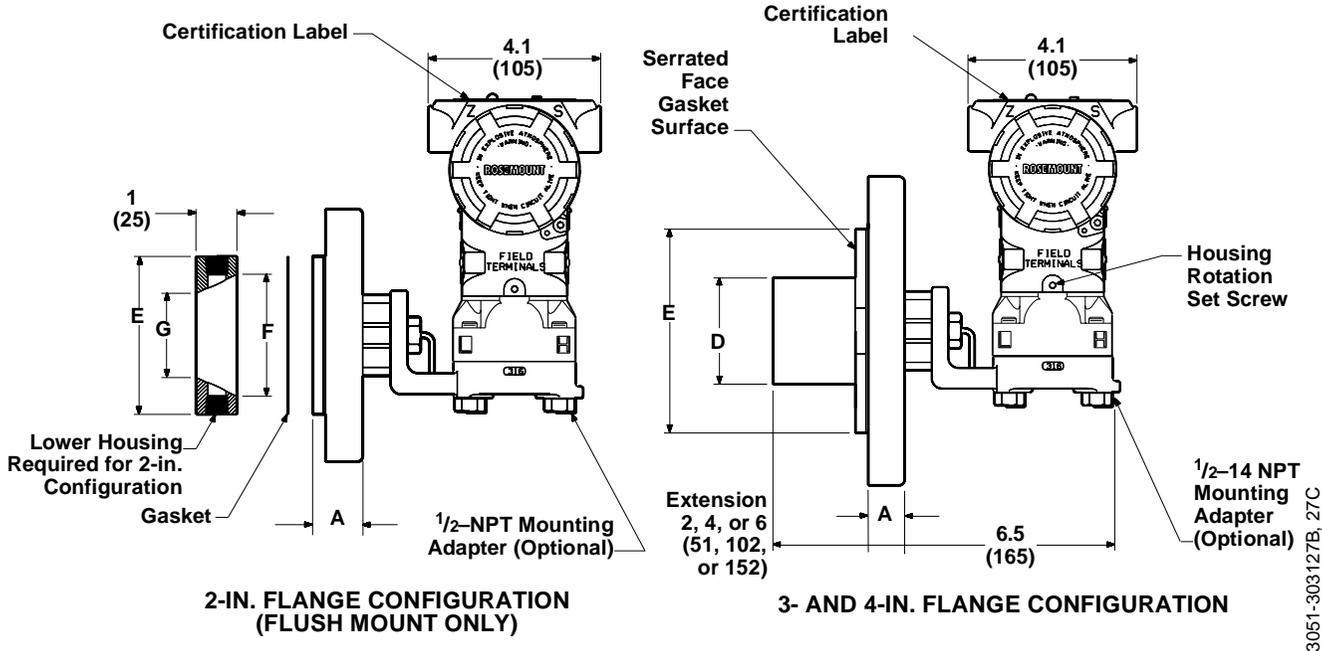
**OPTIONAL FLUSHING CONNECTION RING (LOWER HOUSING)**
