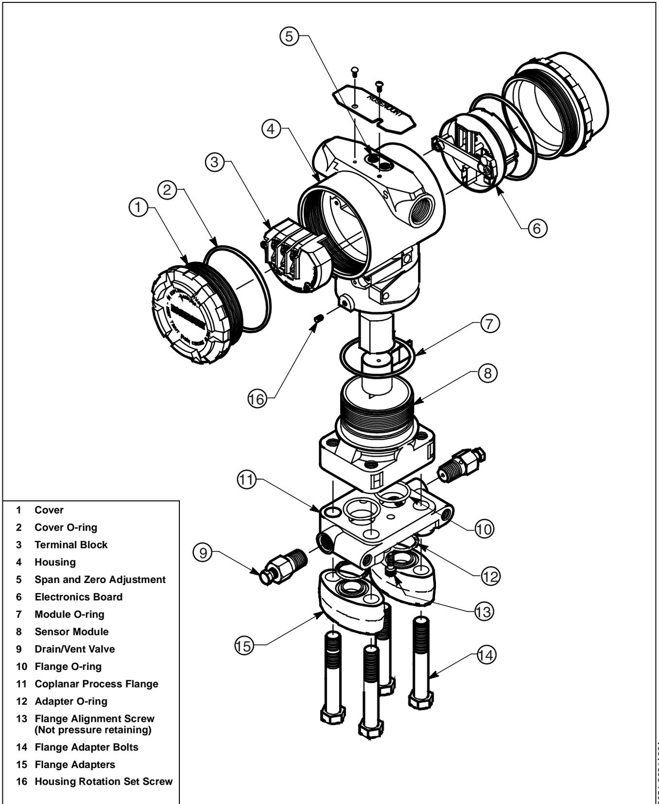
Figure 5-2. Model 3051C Exploded View (with Coplanar Flange).
