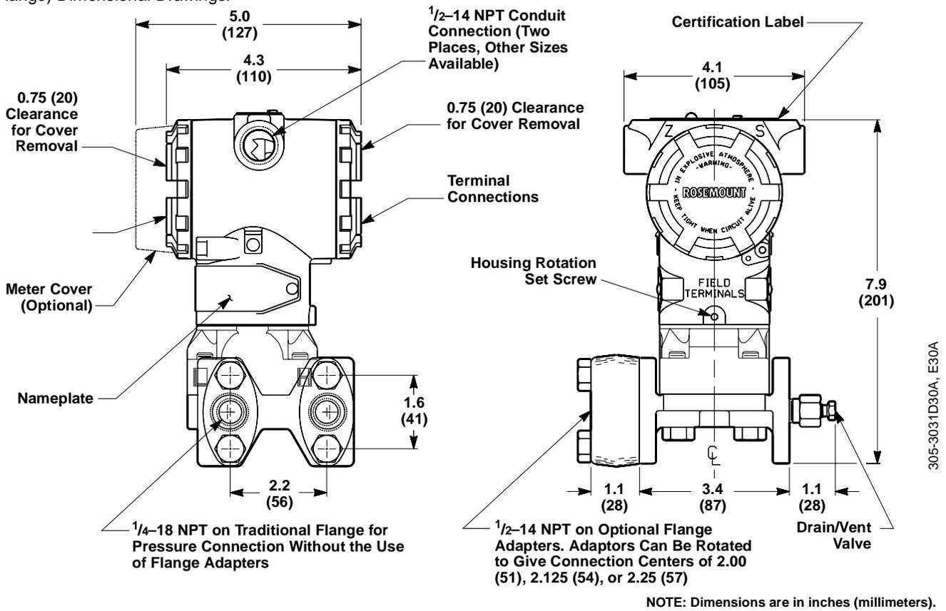
FIGURE 3-5. Model 3051T Dimensional Drawings.
