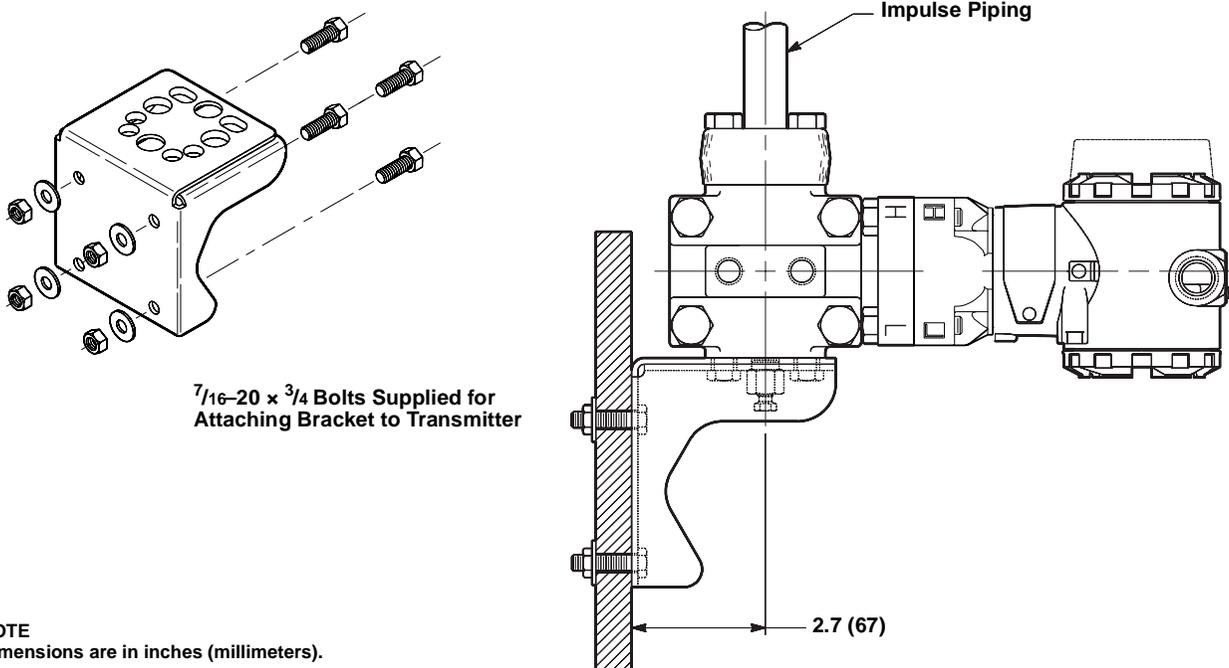
$7/16-20 \times 3/4$  Bolts Supplied for Attaching Bracket to Transmitter
