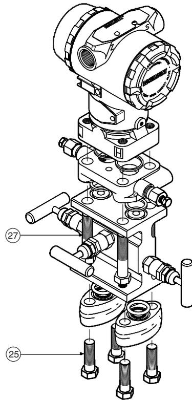
Transmitter with Coplanar Flange and Flange Bolts
