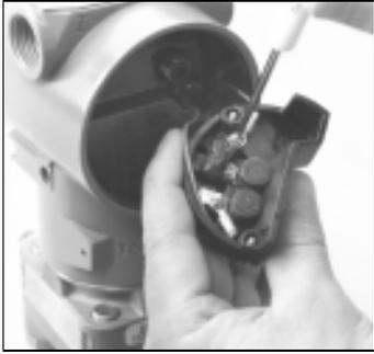
Gently slide the terminal block into place, making sure the posts from the electronics housing properly engage the receptacles on the terminal block. Tighten the captive screws and replace the electronics housing cover. The transmitter covers must be fully engaged to meet explosionproof requirements.
