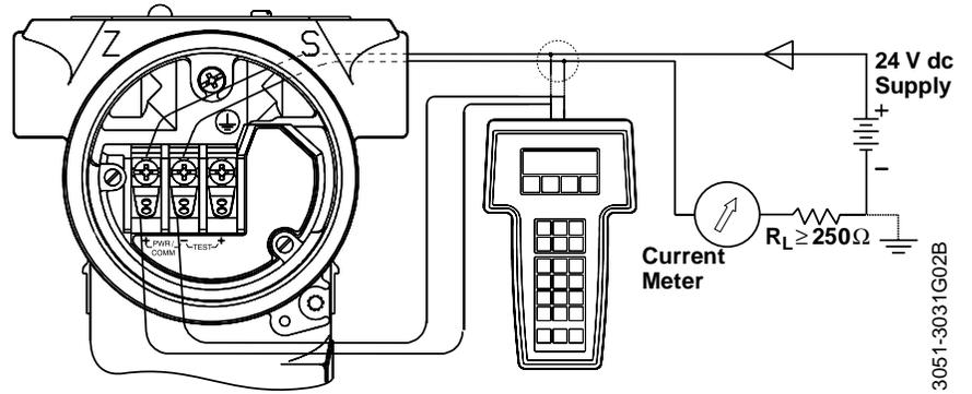
Figure B-3. Bench Hook-up (Low Power Transmitters).
