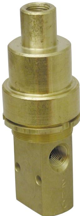
Controlled by a low-pressure signal applied to a small pilot piston integrated into the valve. This actuates the valve. When the pressure is exhausted, the valve returns to the unactuated position. Pilot medium is separate from medium being controlled.
