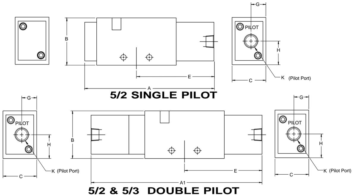
**Dimensions** (See appropriate size series below for locations of mounting holes and ports.)
