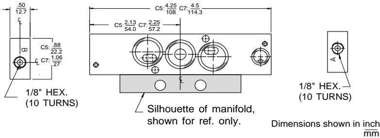
**NOTE: Assembly includes valve mounting screws and O-rings. This product is not available for C7 size EXPilot Valves.**
