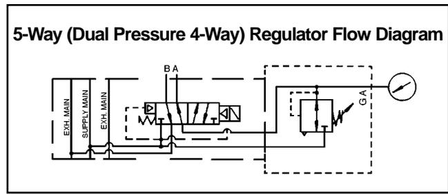
Flow diagram above shows one 5-way single solenoid valve mounted on the regulator assembly. Supply pressure is supplied to 'B' port and regulated pressure is supplied to 'A' port.
