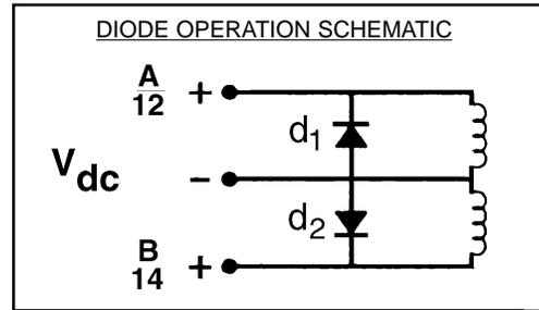
Voltage surge protection (Suffix -SSD) is available in conjunction with the plug-in option on all common DC voltages. Diodes are connected in parallel with the coil and mounted directly to the circuit board providing electrical controllers surge suppression against voltage spikes caused by the solenoid.
