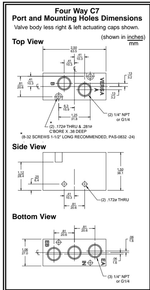
**NOTE:** VALVES SUPPLIED WITH G THREADS HAVE PORTS MARKED AS FOLLOWS: IN=1, A=2, EA=3, B=4, EB=5
