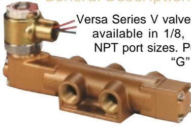
Versa Series V valves are full flow port valves, available in 1/8, 1/4, 3/8, 1/2, 3/4 and 1" NPT port sizes. Ports of 1/8 to 1/2 ISO 228 "G" threads are also available. Three-way designs are provided with 3 ports; four-way designs have 5 ports. Each is available for 2-position or
