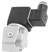
**HC** DIN STYLE COIL & CONNECTOR: DIN type coil with 3 spade terminals and mini-DIN connector with PG9 cord grip. NEMA 4/IP65.
